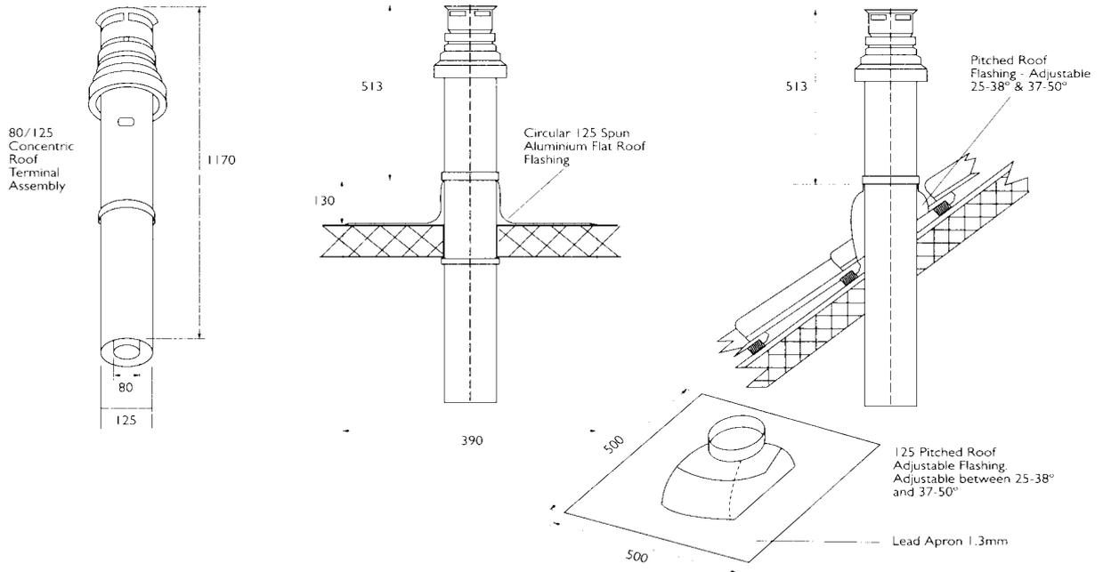
Concentric vertical flue fittings are available from eco hometec.
