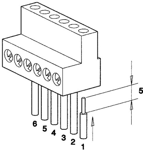
The boiler control inputs are all low voltage and must not be connected directly to the mains.
