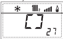
28. Display valve opening control with board MIXED ZONE 2 (respectively ON and OFF)
