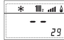
30. Display solar probe temperature value S1 with solar board INSOL
