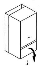
To reach the control panel rotate the small panel as indicated in figure.
