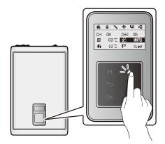
3. Press the OK button (○K) to select the DHW temperature temperature (★1). The highlighted section will flash.
