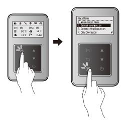
Press the Up button ( $\blacktriangle$ ) or the Down button ( $\blacktriangledown$ ) to switch between the information items. Press the OK button ( $\bigcirc$ K) to select an item and view the information.
