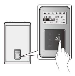
2. Press the OK button (○K) to select the space heating temperature (Ⅲ). The highlighted section will flash.
