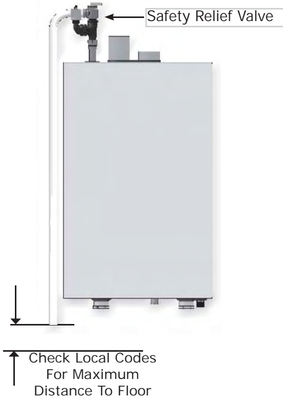
FIGURE 5-2 Safety Relief Valve Discharge Piping
